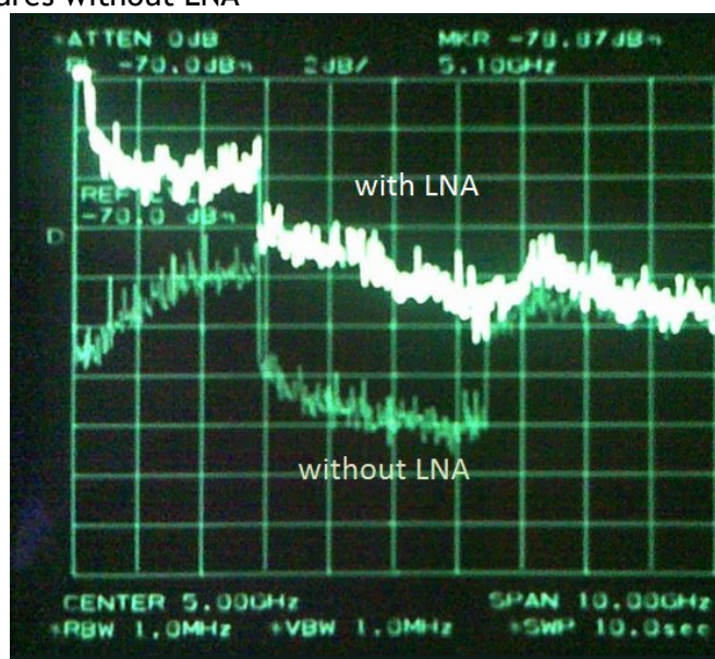
Figure 2: Noise floor versus frequency of spectrum analyzer preceded by LNA.
