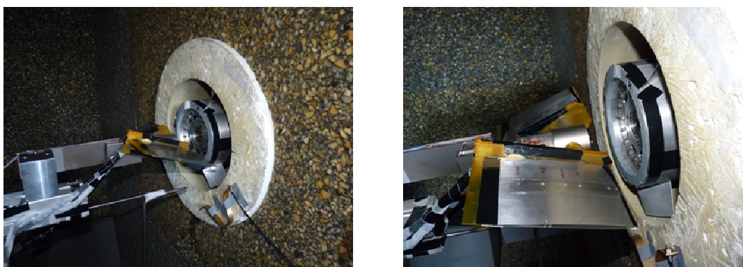
Figure 1. Rotor, airfoil and balance general view (left) and airfoil detailed view (right).
