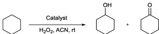
Scheme 2. Oxidation of cyclohexane into cyclohexanol (OH) and cyclohexanone (=O).
