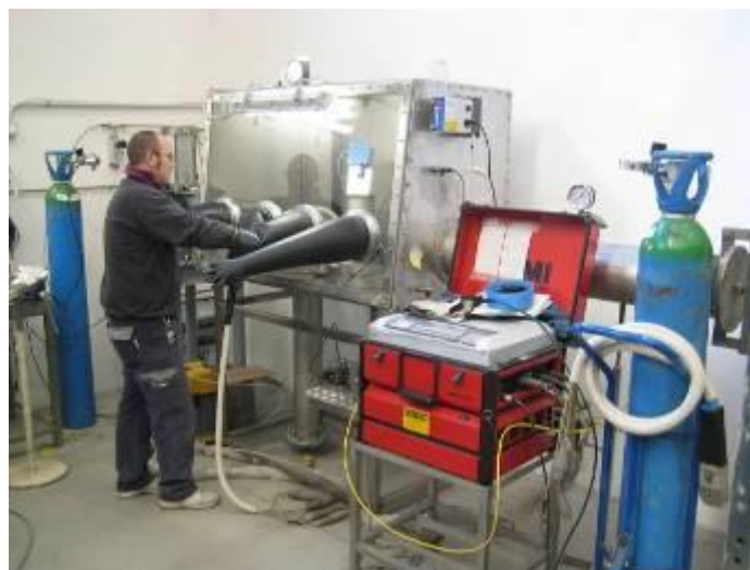
Figure 20: Orbital welding inside of the glove box
