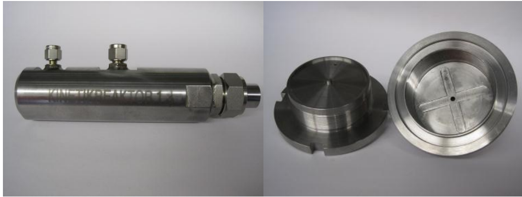
Figure 11: Reactors used for measurement of effective rate of reactions at different temperatures and pressures. Left: CxH material. Right: MeH material.
