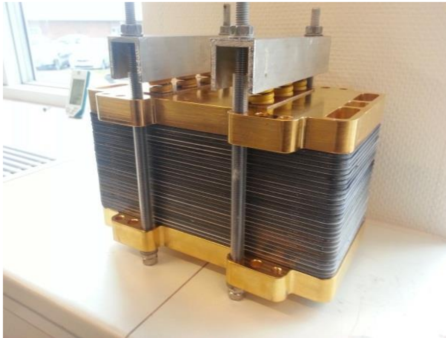
Figure 25: 25 Cell, 163.5 cm 2 liquid cooled stack - 1kW - Operation temperature 120 -170 °C.
