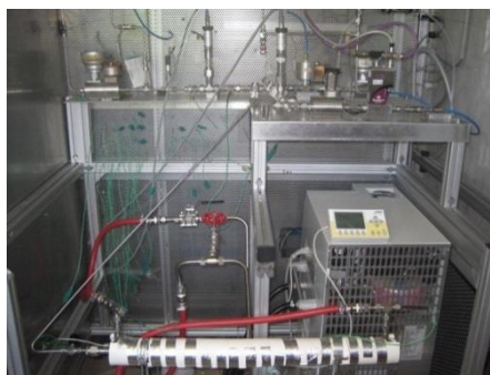
Figure 22: Experimental setup with insulated tank in front and thermostatic bath on the right.
