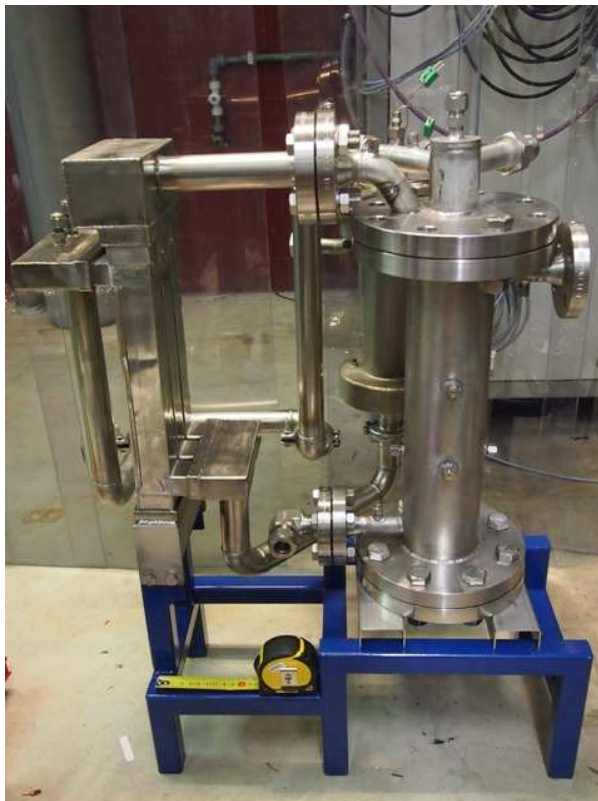
Figure 21: Assembly of the reformer burner, Air preheater and steam generator
