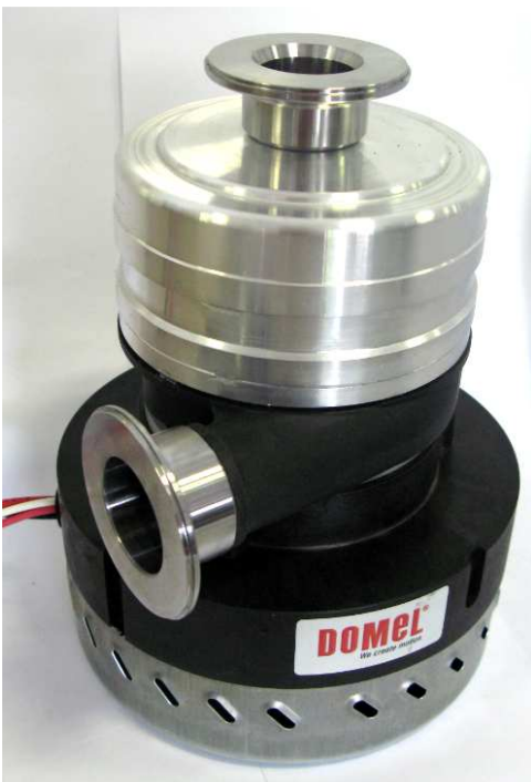
Figure 23: Three stage GAD system prototype No.1 with integrated electronics
