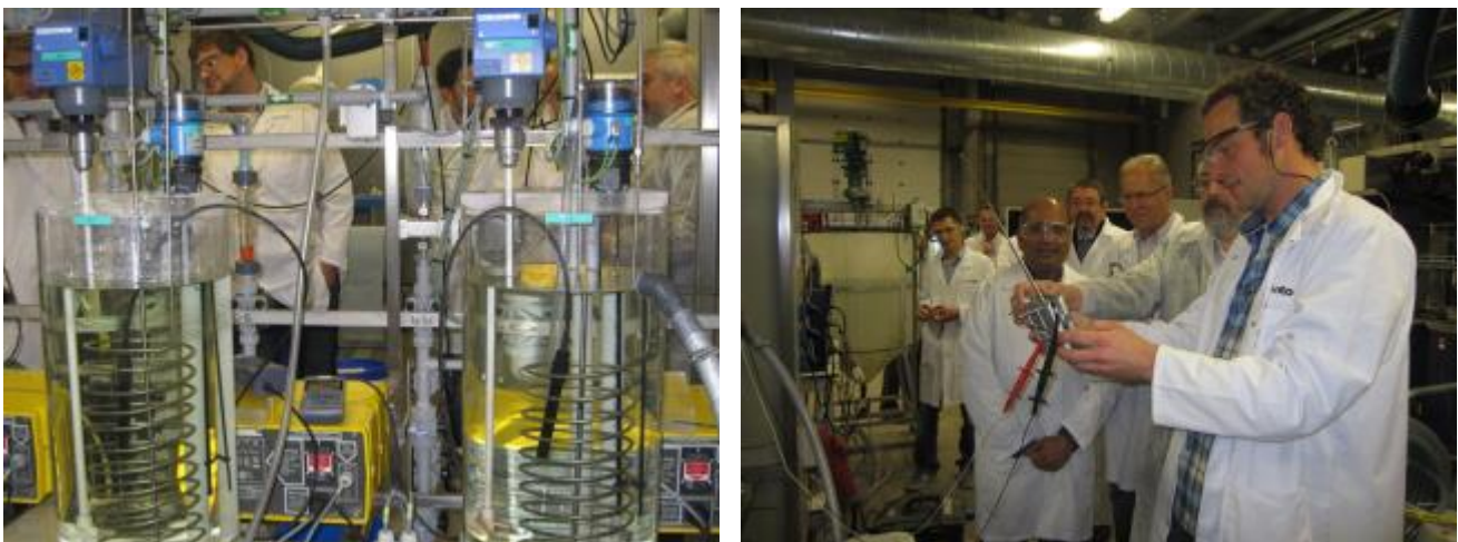
The lab stack is tested at the lab of VITO and is used to operate a radio during the visit of the REAPower team and the EC representatives.
