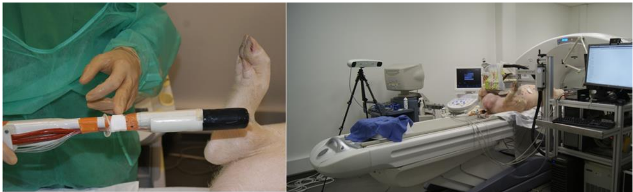
Fig. 1: Left) Optimized final version of the EndoTOFPET-US probe. The probe was found to be usable under the clinical practice for prostatic investigations and clinicians approved the design of the prototype. The probe was optimally placed in-situ according the ultrasonic imaging of the prostate. Right) Arrangement of the whole EndoTOFPET-US system within a standard examination room.
