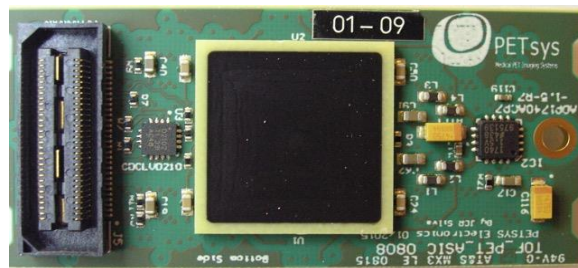
Fig. 8: The TOFPET FEB/A board with 128 channels (two ASICs under the common globtop protection epoxy).
