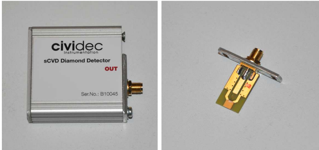
Large area CIVIDEC diamond detector.
