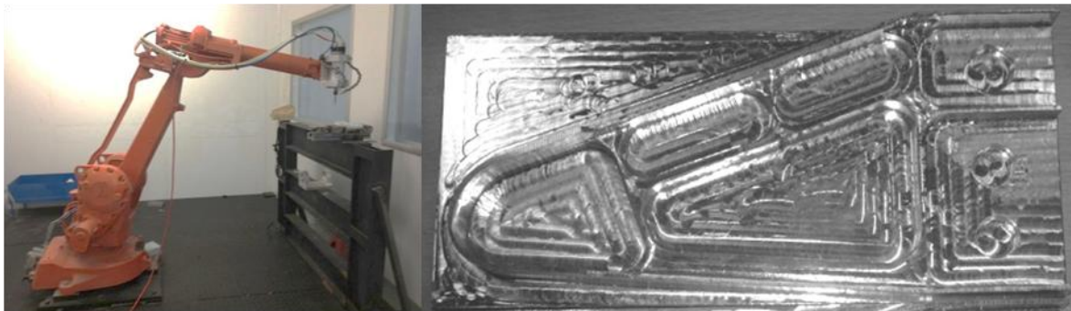
Figure 3.6-1 left: TEKS COMET cell; right: Aluminium wing's component machined by robot
