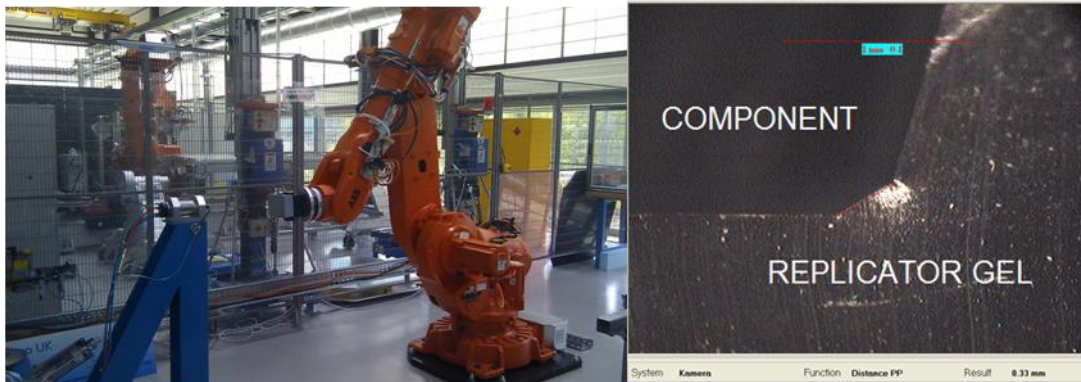
Figure 3.6-2 left: AML COMET cell; right: microscope image of deburred edge of test part feature
