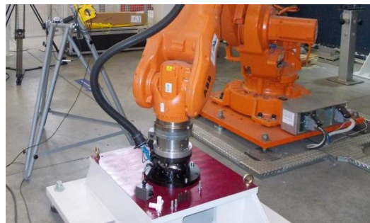
Figure 3.1-3: Joint parameter identification using the Clamping Method at project partner SIR
