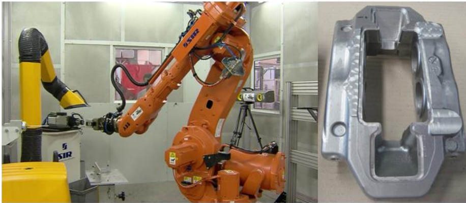
Figure 3.6-3 left: SIR COMET cell; right: cast brake calliper machined by robot (chamfered)
