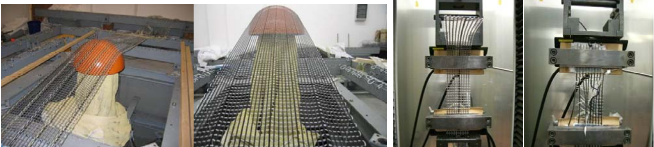
Figure 3.43: Examples of testing procedure: net test (left) and tensile strength (right)
