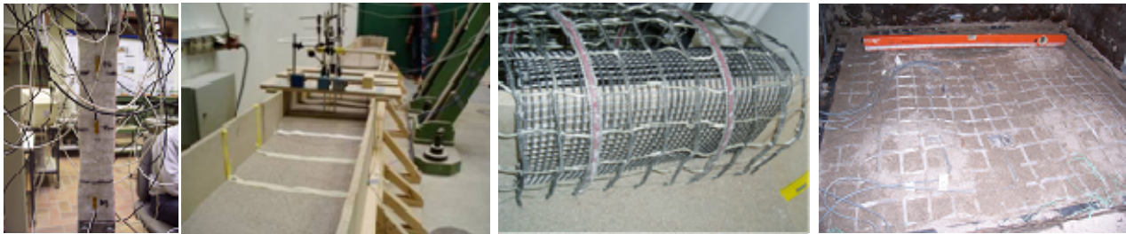
Testing of a filter mat, the “long box” test, SMARTeC smart profile geogrid, and the “square box” test at Uni-Kassel
