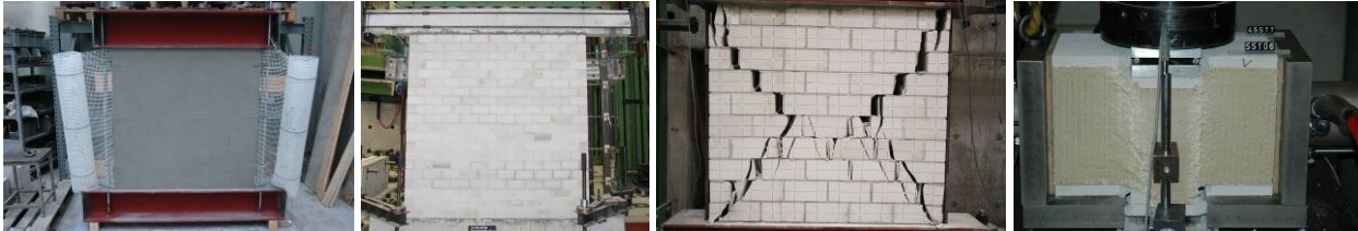
Laboratory tests on small scale and large scale textile reinforced masonry walls at the University of Karlsruhe, Germany and at CETMA, Italy
