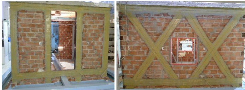
Figure 3.52: IMG strips reinforcement by multifunctional uni-axial textile
