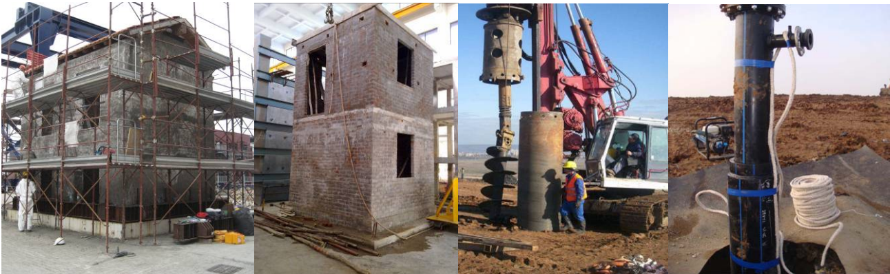
Polytect 4 th Year Field Tests: Shaking table test of stone masonry building (Italy), of brick masonry building (India) and test of rope like structures with chemical sensors in a landfill (Romania)
