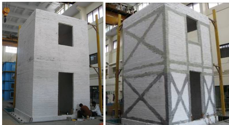
Figure 3.53:IIT Madras masonry building: un-reinforced (left); strips reinforced (right)
