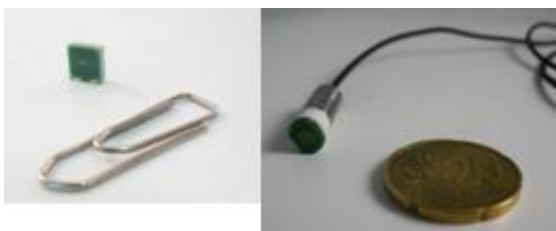
Figure 50: Eddy Current Sensors (ECS) integrated into the Generator
