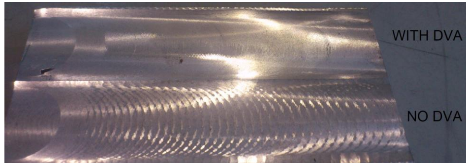
Figure 27: Cutting conditions and workpiece surface after machining, with and without DVA
