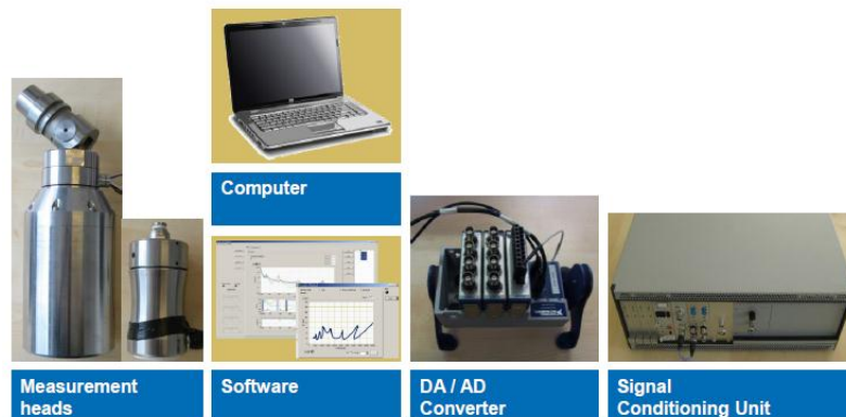
Figure 39: Components of dynamics calibrator.
