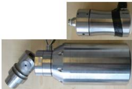
Figure 4: HPC (left) and HSC (right) dynamics calibrators.
