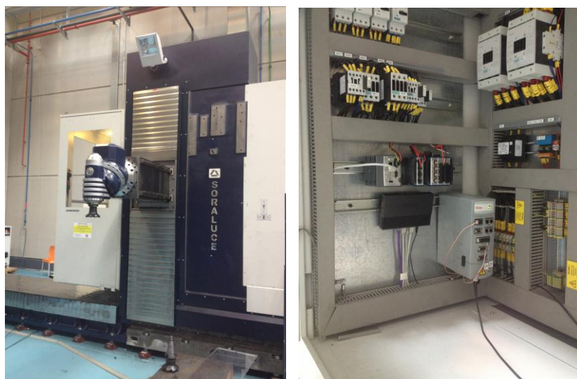
Figure 10: Integration of the actuator and the control system on the FL6000 milling machine.
