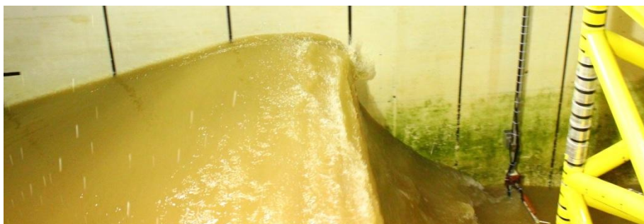
Figure 3.9 Focussed wave generated using self-correcting method in shallow water in front of a truss structure (courtesy of LUH)
