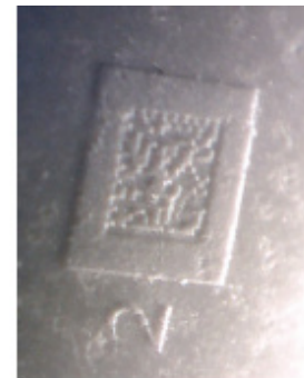
Code 2 at the end of the run (stamped on a hard tablet)
