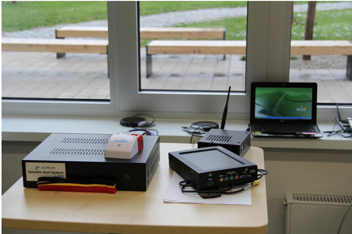
Figure 3-40: DVB-SH to portable devices (sirens)
