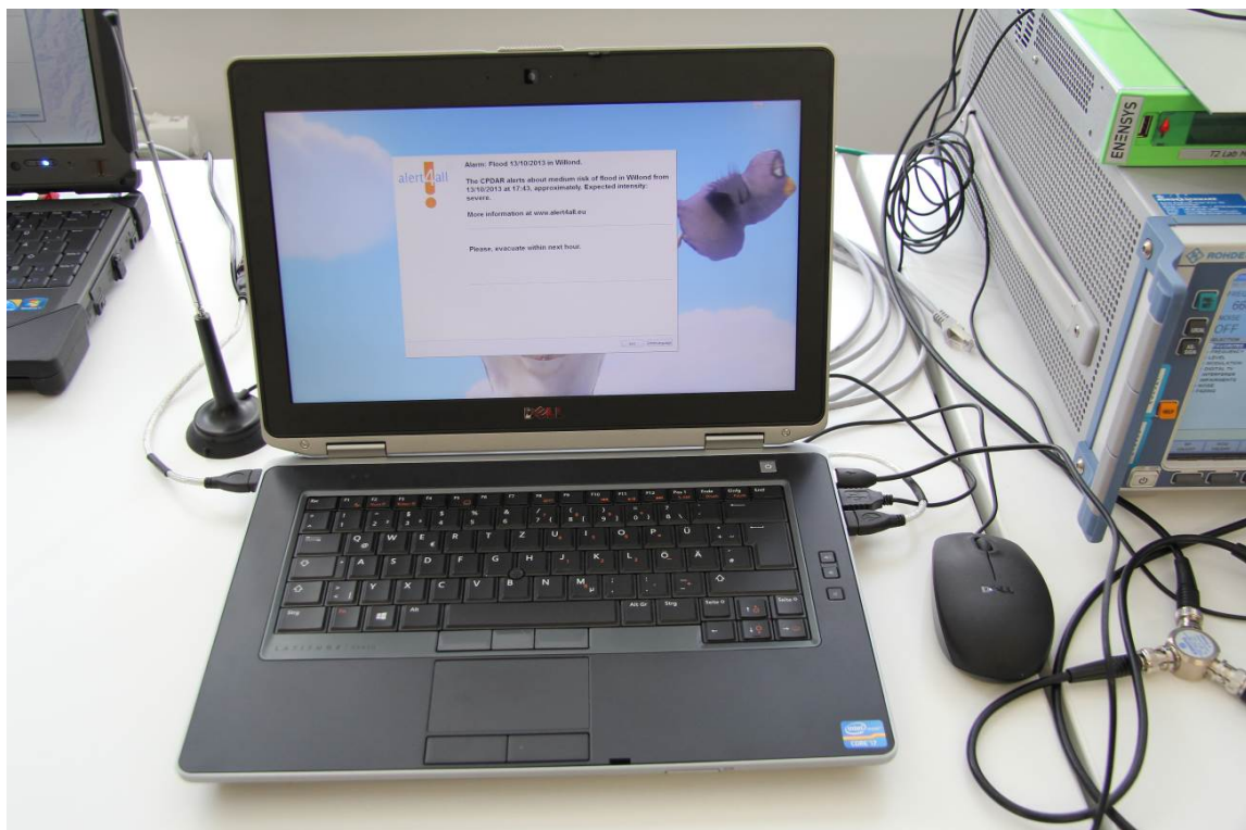
Figure 3-37: Alert delivered over enhanced DVB-T2 receiver
