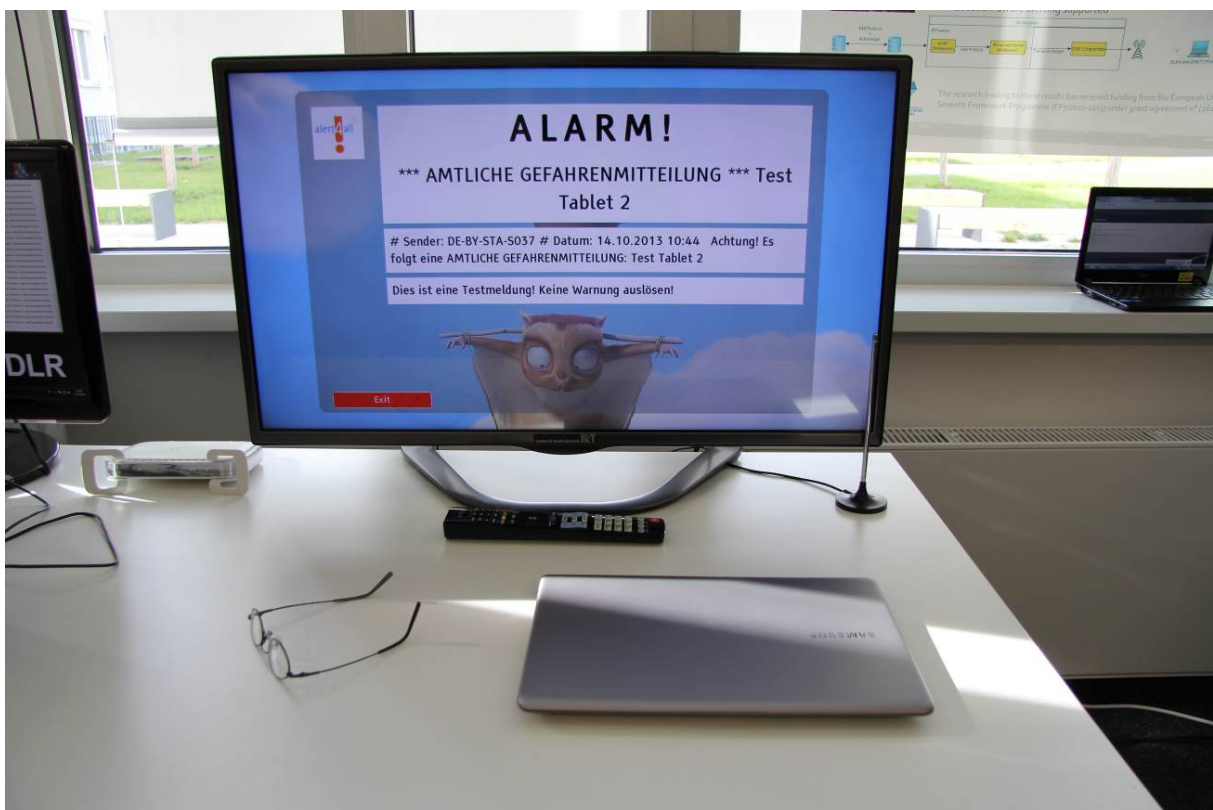
Figure 3-35: Alert delivered over HbbTV (terrestrial)
