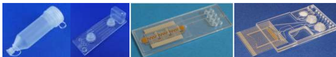
Figure 13: Sampling vessel (left), immunoassay module (second from left), hybridization module for electrochemical assay set-up (third from left) and immunoassay chip for electrochemical detection (right)
