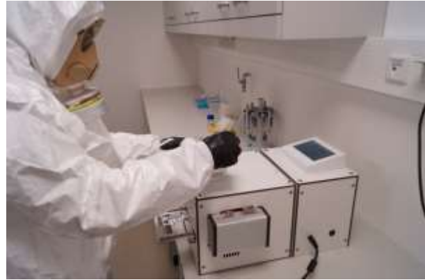
Figure 33: End-user testing the handling of the OTM consumable wearing the protective suit
