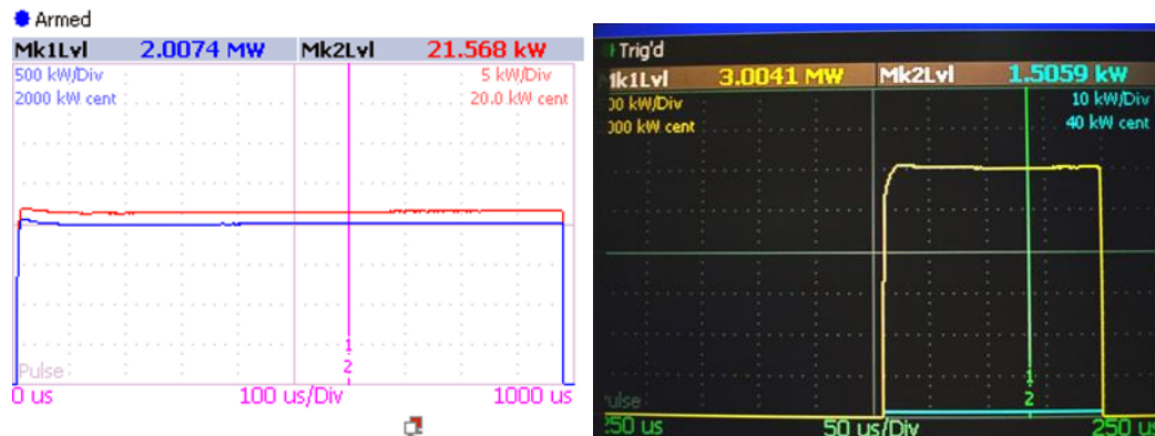
Figure 7.8: Illustration of the pulse envelopes achieved with the diacode based power amplifier, on the LHS demonstrating the current ICTF specification pulses at 1Hz PRF and on the RHS showing the peak performance of the amplifier at 3MW.
