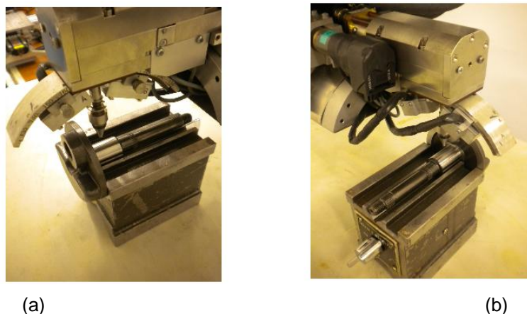
Figure 22: XRD measurement: (a) Axial direction; (b) Circumferential direction.
