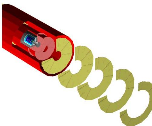
*Figure 1: Inner tracking detectors (VXD, SIT, FTD) of the ILC detector concept for the ILC in a DD4hep based geometry model.*
