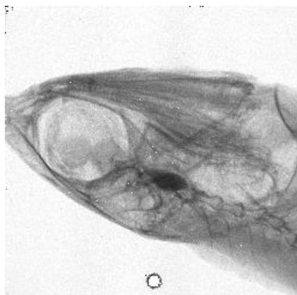
Figure 11: An X-ray image (flat field corrected) of a small fish head taken using a TSV-processed Medipix3 chip which has been flip chip bonded to a Silicon sensor. The chip has 256 x 256 pixels on a pitch of 55 $\mu$ m. The readout is performed through the BGA contacts on the back of the ASIC. The origin of the circular artefact is not known
