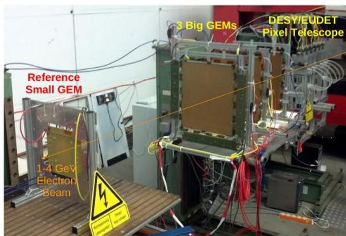
Figure 16: View of experimental set-up at DESY using pixel telescope
