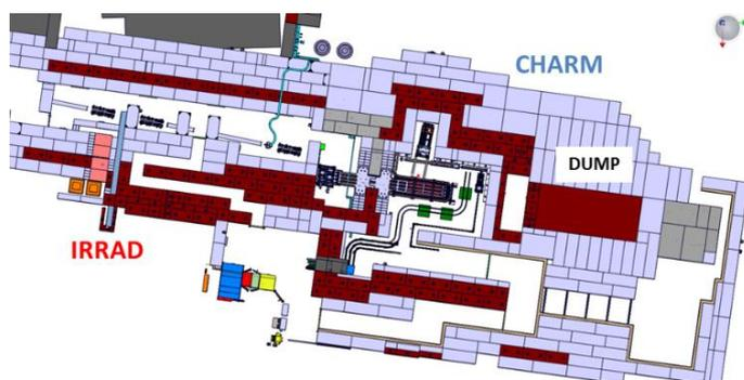
Figure 23: Layout of the new combined EA-IRRAD facility implemented on the T8 beam-line: the proton area, IRRAD (upstream), is followed by the mixed-field area CHARM (downstream).
