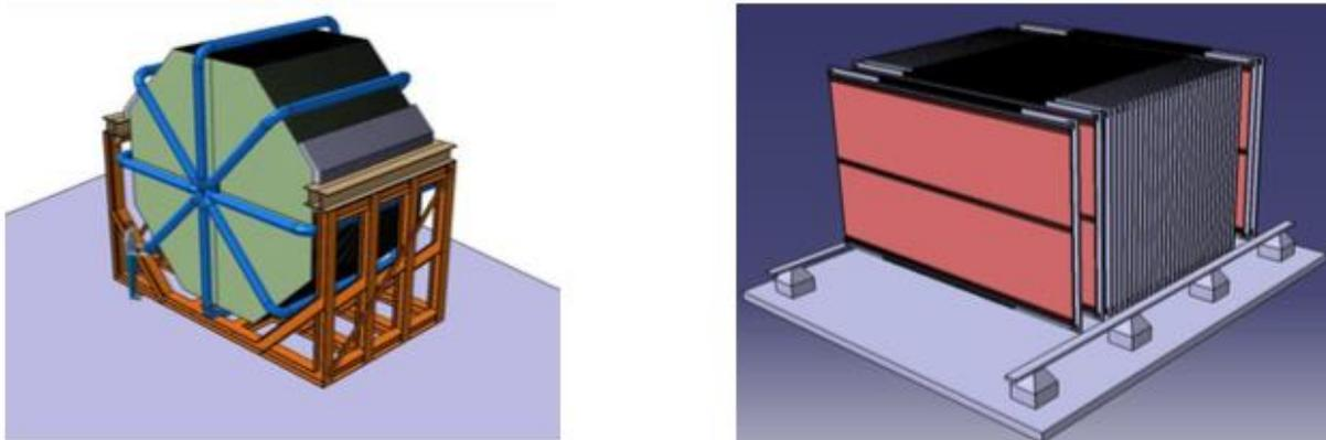
Figure 30: Left) Traditional approach to MIND magnet design, with one or more transmission lines around all iron plates. Right) New design proposed for the AIDA MIND where every individual iron plate has its own coil windings, leading to increased modularity and flexibility in choosing optimal separation gap between plates.
