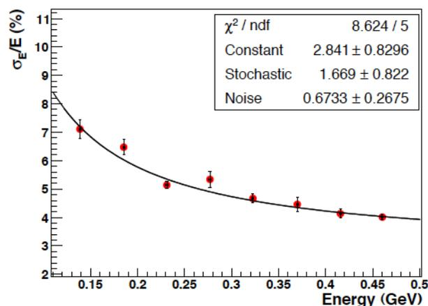
Figure 22: Measurements of LYSO energy resolution for the characterisation of the Frascati test beam. SiPM readout is used.
