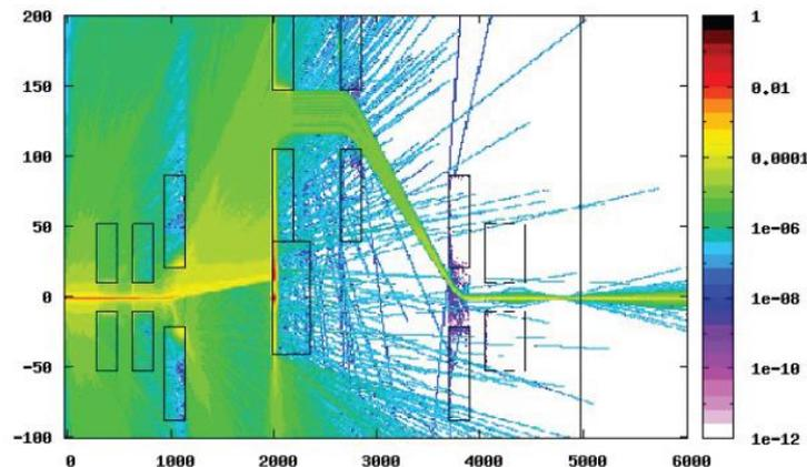
Figure 20: Particle trajectories with the same layout for a low energy electron beam of 9 GeV/c.
