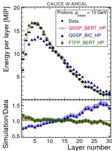
Figure 41: Longitudinal shower profile for 10 GeV protons in a Tungsten calorimeter stack.
