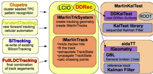
Figure 5: Schematic view of new ILD tracking software where the pattern recognition algorithms are programmed against the *IMarlinTrk* interface and thus independent of the actual track fitting algorithm used.
