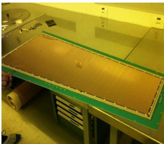
*Figure 33: Large area GEM muon chamber prototype for the CMS experiment*
