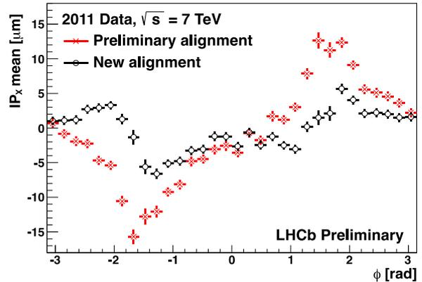
Figure 8: Mean of Impact Parameter versus the azimuthal angle for LHCb data events using old and new alignment procedures of the VELO detector that correct for weak modes.
