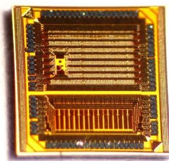
Figure 40: 8-channel ADC ASIC for forward calorimeters.
