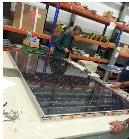
*Figure 32: Photo of a large cosmic ray telescope chamber during assembly.*
