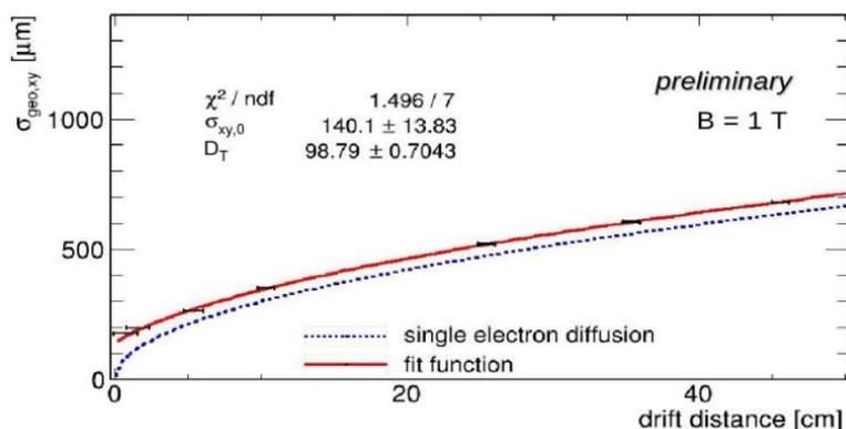
Figure 35: Spatial resolution versus drift distance measured in a beam test in the large TPC test infrastructure at DESY compared to the expectation limit given by diffusion.
