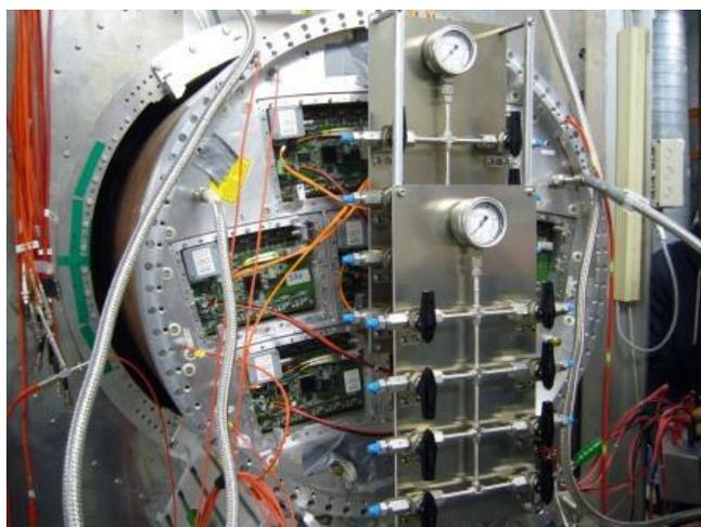
*Figure 34: The PCMAG endplate instrumented with micromegas readout at the DESY TPC facility.*
