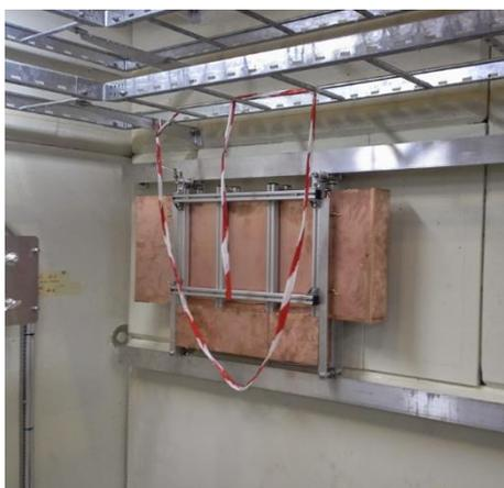
*Figure 31: Doublets of TGC's mounted in the front part of the GIF++ facility. The front end electronics is covered by the Faraday cages. The tracker is mounted on rails so that it can be moved out of the beam-line.*
