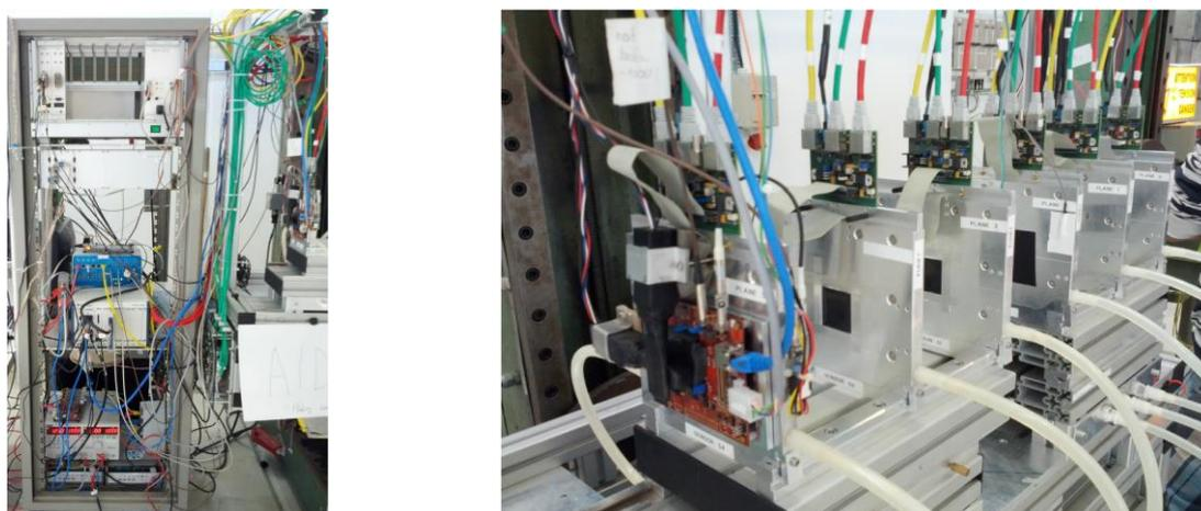
Figure 36: Commissioning of the AIDA telescope in July 2014 in the CERN PS T9 beam line: (left) The AIDA telescope rack contains (top-to-bottom) DCS, TLU and miniTLU, NI readout for Mimosa26 sensors. USBPIX readout for FEI4 module on top of the three channel TTI power supply and power supplies for Mimosa sensors and electronics. (right) The photo shows an upstream look at the telescope sensor planes with the FEI4 plane being mounted as the most downstream plane (on the left of the picture).
