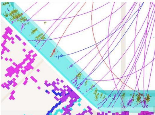
Figure 9: Particle flow objects (PFOs) reconstructed by PandoraPFA in the ILD detector: charged particles (dark blue); photons (mustard yellow); electrons (red) and neutral hadrons (light blue).
