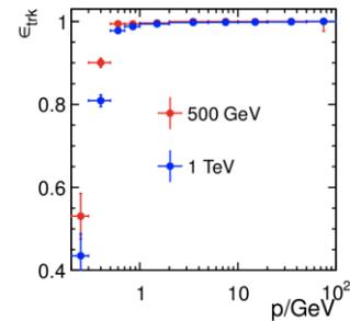
Figure 6: Track finding efficiency for prompt tracks in *ttbar* events at the ILC with 500 GeV and 1 TeV center of mass energy respectively, as a function of momentum.
