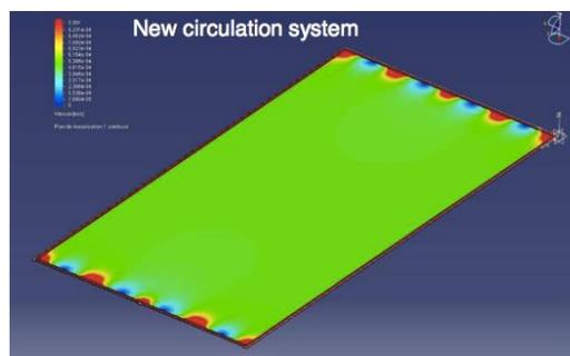
Figure 39: Mechanical simulation of  $2 \times 1$  m<sup>2</sup> chamber showing effect of new gas circulation
