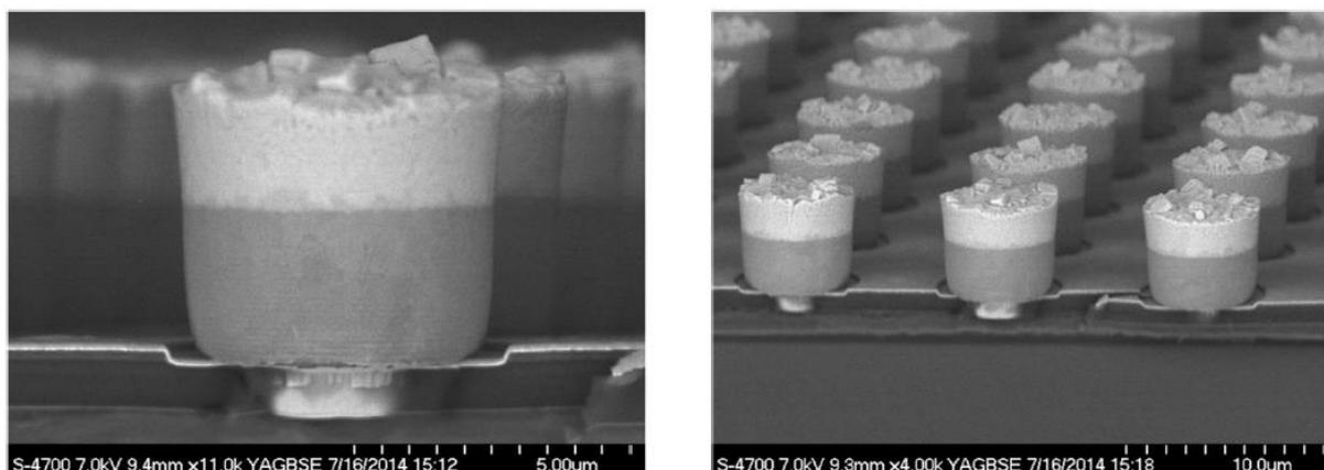
Figure 12: Images of bumps for the SLID interconnection at IMS for the sub-project. The diameter of a bump is 5  $\mu$ m, the pitch 10  $\mu$ m.
