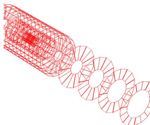
*Figure 2: Measurement surfaces attached to the sensitive detector elements used for track reconstruction.*
