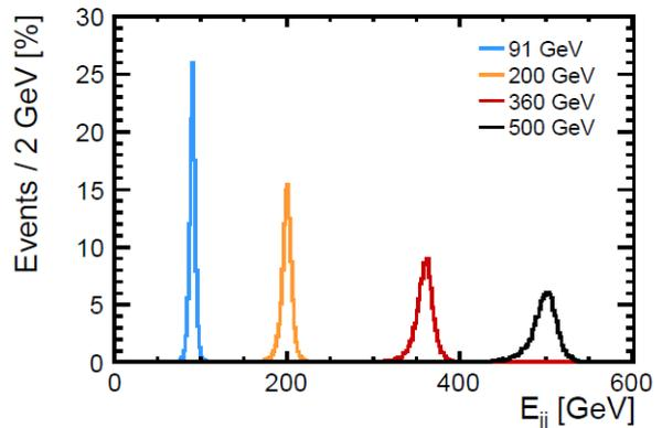
Figure 10: Total reconstructed di-jet energy distributions for  $Z \rightarrow uu/dd/ss$  at various center of mass energies.
