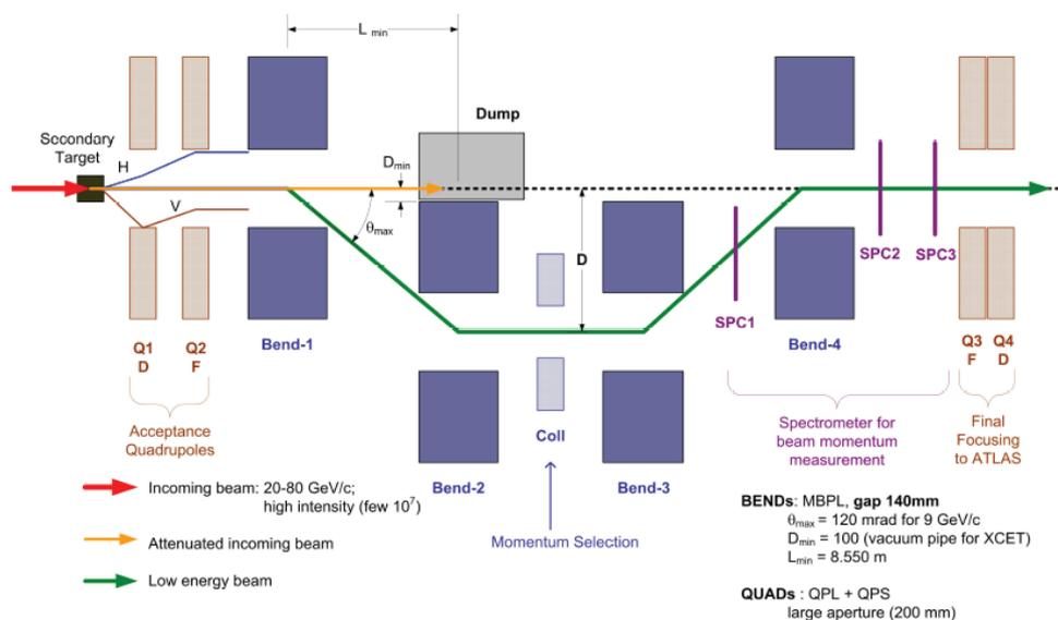
Figure 19: Schematic of beam layout for very low energy beam in H8.
