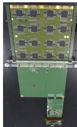
*Figure 37: PCB with ASICs for 18×18 cm<sup>2</sup> Si-W ECAL.*
