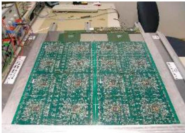
Figure 38: Electronic board for analogue HCAL prototype.
