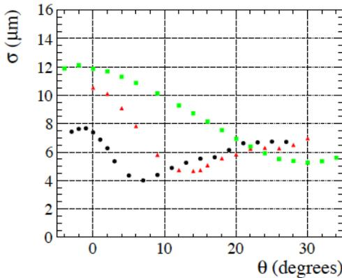
Figure 7: Resolution versus track angle at 60V bias voltage for 150 $\mu\text{m}$  (green) 200 $\mu\text{m}$  (red) and 300 $\mu\text{m}$  (black) thick prototype Silicon pixel sensors with TimePix ASIC using the BACH alignment software and the TimePix telescope.
