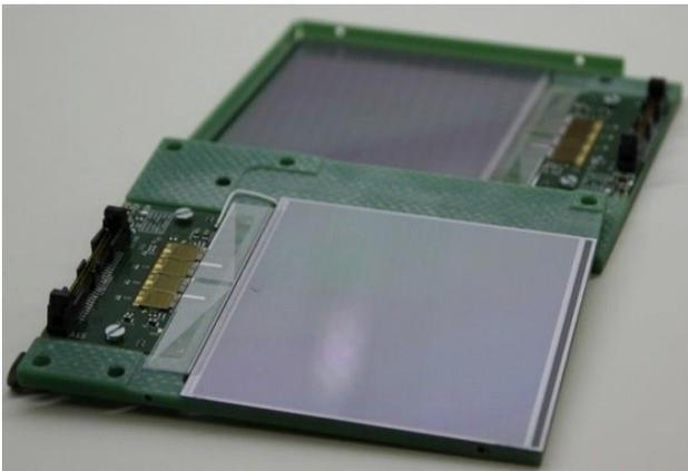
Figure 43: Micro-strip sensors used to construct the mini-telescope.
