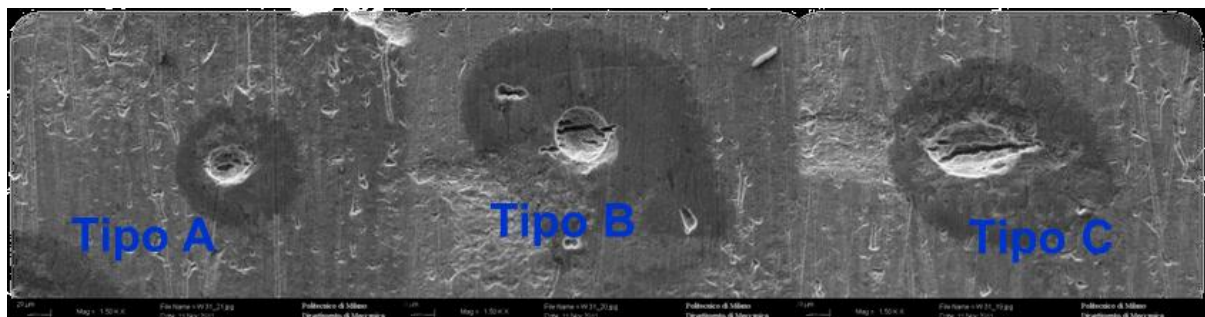
Figure 7 Growth of Crack within a pit
