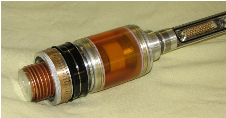
Figure 25 Phased array probe developed in project
