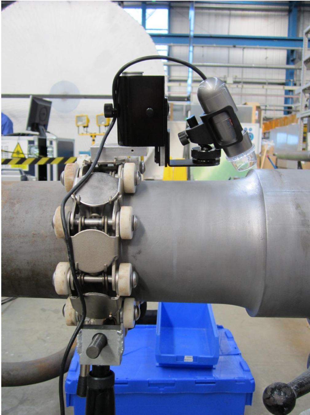
Figure 10 Microscope, holder and scanner for corrosion assessment
