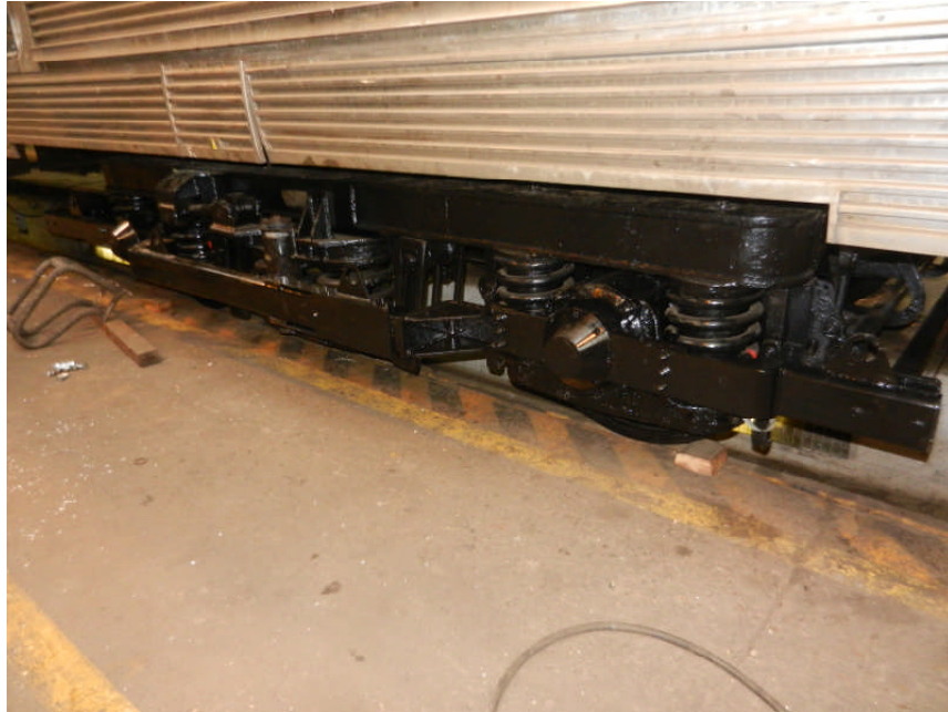
Figure 19: Deployment mechanism frame installed on the bogie of the test train.
