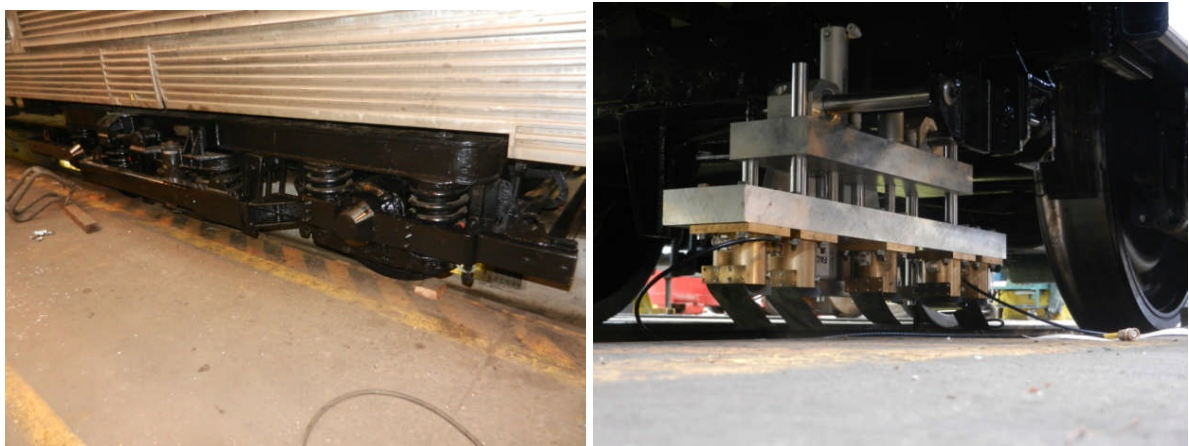
Figure 3: Deployment mechanism frame installed on the bogie of the test train.
