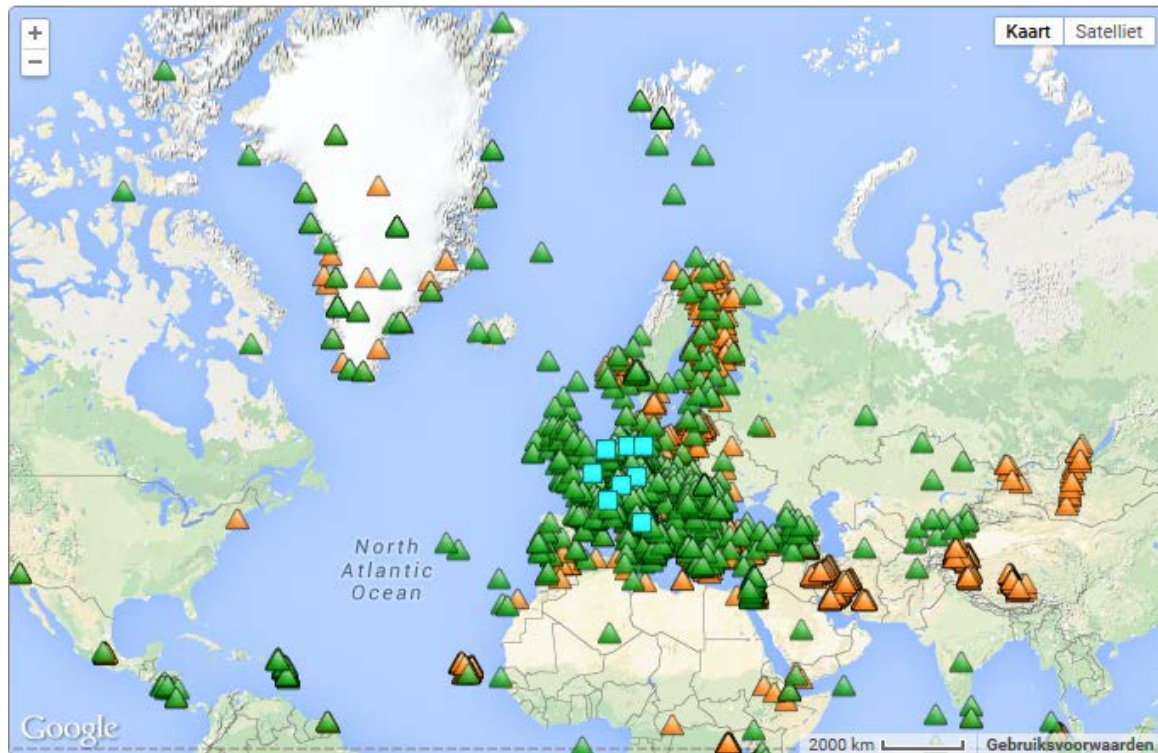
Figure 1 – geographical distribution of seismic stations in and around Europe from which data is openly available through the distributed, federated data archive (EIDA; www.orfeus-eu.org/eida ). Green triangles are permanent seismic stations, orange triangles are temporary stations and blue squares are the connected data archives.
