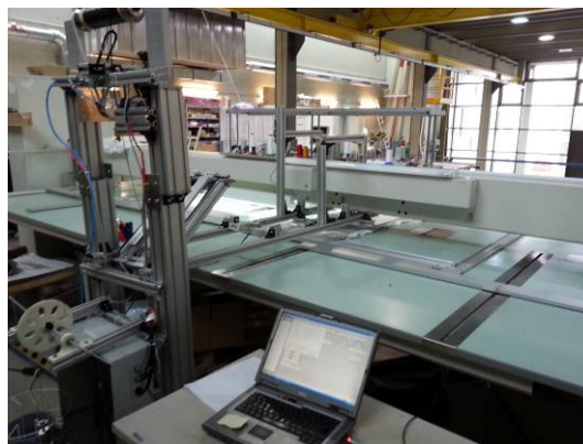
Back view of the TFP machine with the developed external feeding device
