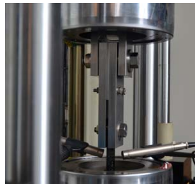
Figure 15.- Experimental setup – special fixture was used for testing the bearing strength of the samples. The microphones on either side were used for acoustic measurement
