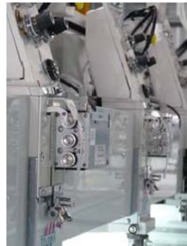
Thread tension measurement device adapted at the TCWM machine
