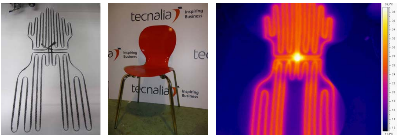
Figure 17.- Manufactured self-heated outdoor chair
