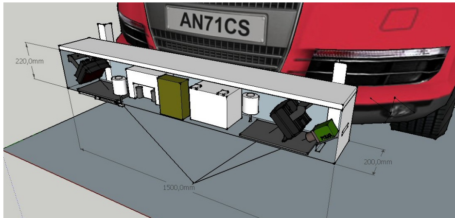
Principle of camera mounting on a vehicle. All sensors integrated into a single housing.
