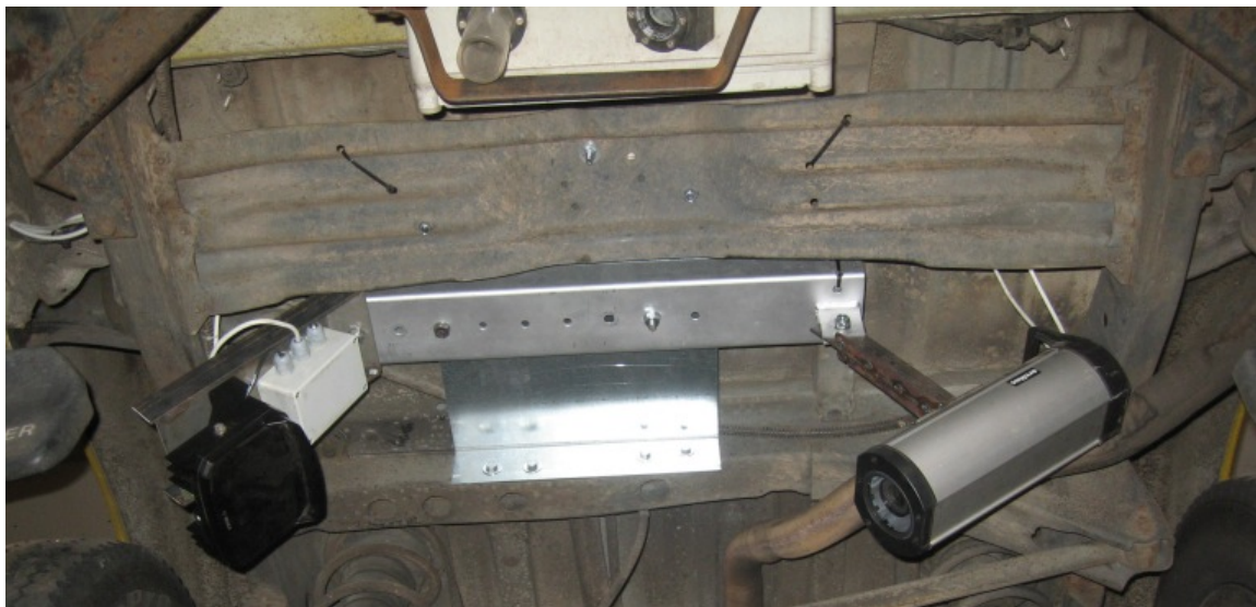
Mounting of IR-source and camera during field tests.
