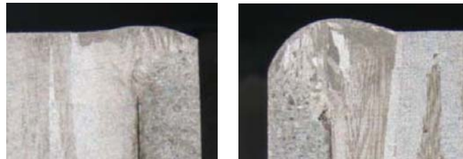
Figure 13: Cross section of nickel joint welded at 2m/min (left) and at 1,5m/min (right)
