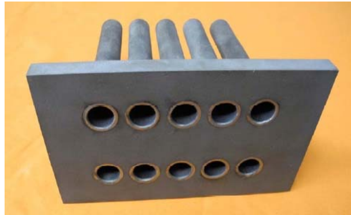
Figure 10: Demonstration sample welded after alignment and calibration of the ORBITAL head
