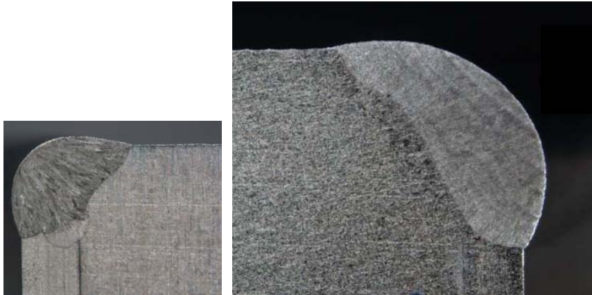
Figure 15: Metallographic cuts of Stainless steel samples welded by LASER (left) and TIG (right)
