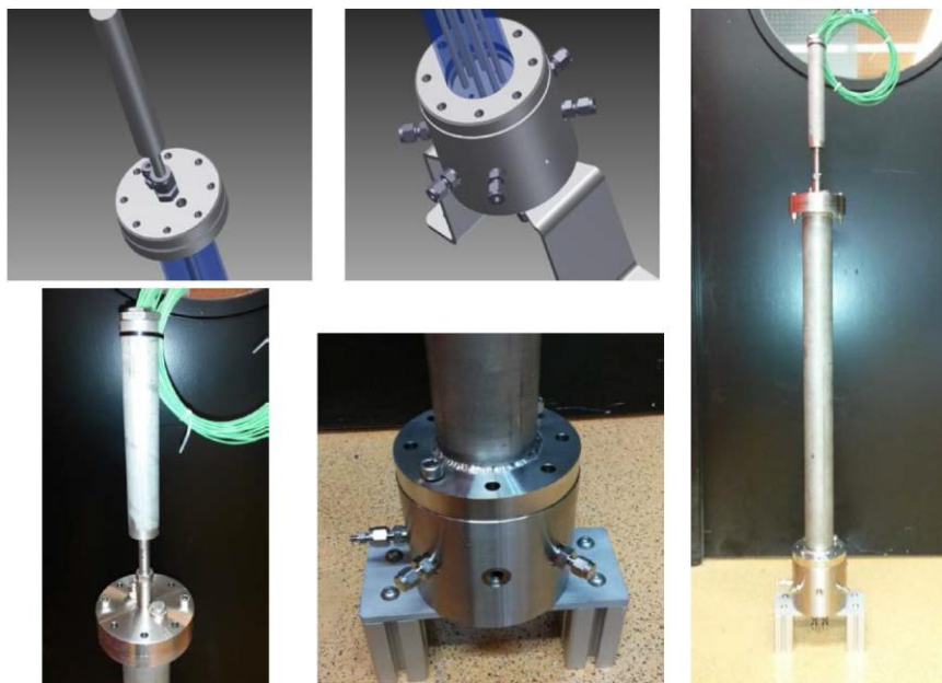
Figure 17. Parts of the new reactor as designed and built and final reactor assembled.
