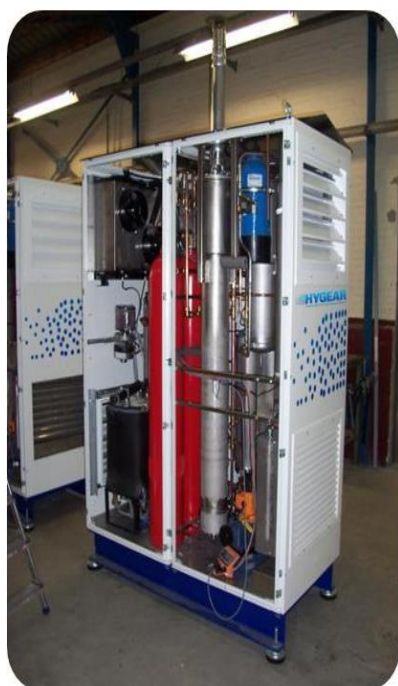
Figure 34. HyGear's (HT&S) on-site hydrogen generation systems: Left: 5 Nm 3 /h system ; Right: 50 and 100 Nm 3 /h system
