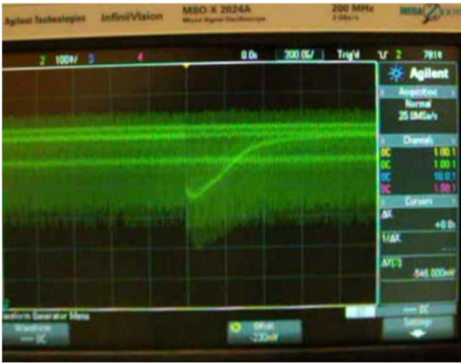
Figure 25. Left: screen capture of the real-time signal traces when the TDM circuit is operated in 4-pixel mode and one pixel captures an X-ray event. The 'hair' in picture are glitches at the time slot edges, which are decimated away from the histogrammed data. Right: an energy histogram showing the 5.9 keV \alpha -complex of the 55-Fe source.
