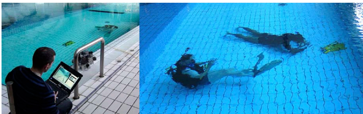
Tests of the teleoperation of the ROV via the internet
