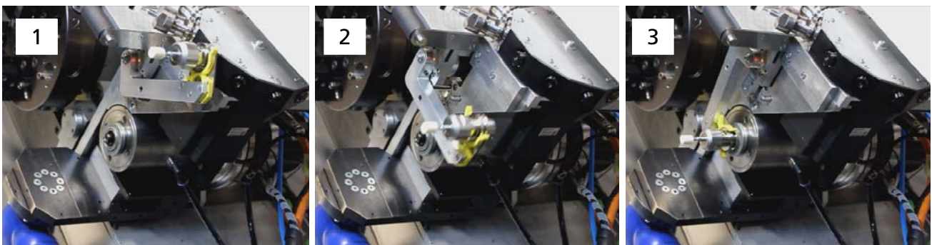
Figure 3: Automated polishing tool change
