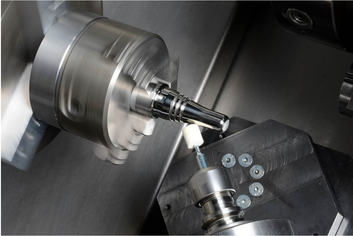
Figure 2: Polishing of a workpiece right in the turning machine
