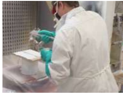
UV coating spray coated with a low pressure high volume gun
