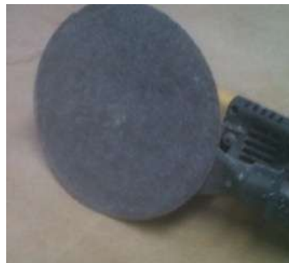
Clean sanding disc to demonstrate that the upper surface is fully cured
