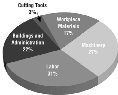
Figure 1: Machining cost and impact of a 20% increased cutting speed with high quality tools
