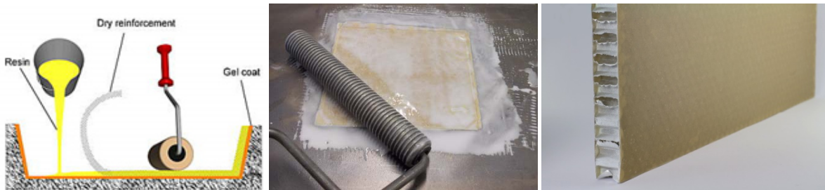
Figure 6.1 Hand layup using nanocellulose sheets from WP5.
