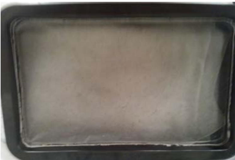
Figure 5.1 Sheet of nanocellulose and modified xyloglucan dried for 120hrs in drying chamber.
