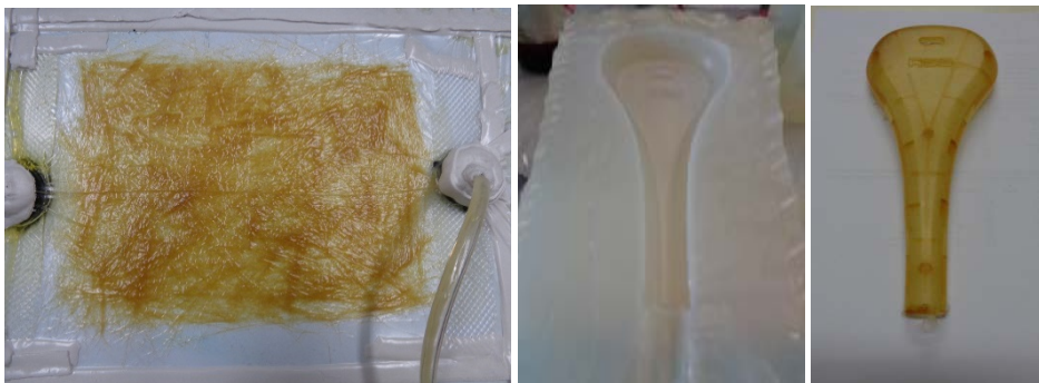
Figure 6.2 Vacuum bagging (left) and resin transfer (middle and right) using nanocellulose fibres from WP5.
