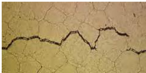
Figure 45: Interface crack in PP-Ni.
