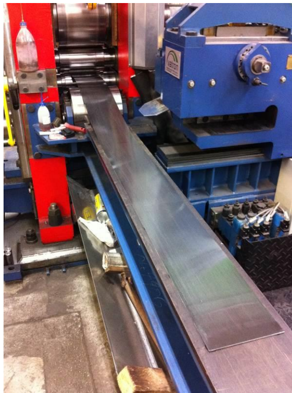
Figure 6: Finishing of cold rolling process, material in hardened condition.
