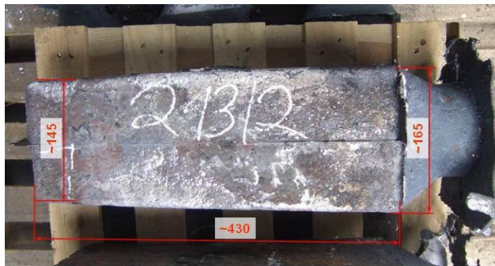
Figure 3: Nb-containing ingot after casting (~90kg).
