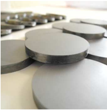
Figure 32: Demonstration of synthesis (3kg batches) and sintering scalability of the host matrix processes developed with NEAT : 60mm diameter pellets sintered by SPS of P-type \text{Si}_{0.8}\text{Ge}_{0.2} host matrix alloys (left) and, N-type \text{Mg}_2\text{Si}_{0.4}\text{Sn}_{0.6} (right)
