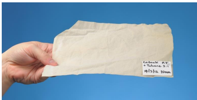
Figure 8 Photograph of cotton textile impregnated with a triple functional silsesquioxane/copper nanoparticle and cured at 120°C for 5 minutes.
