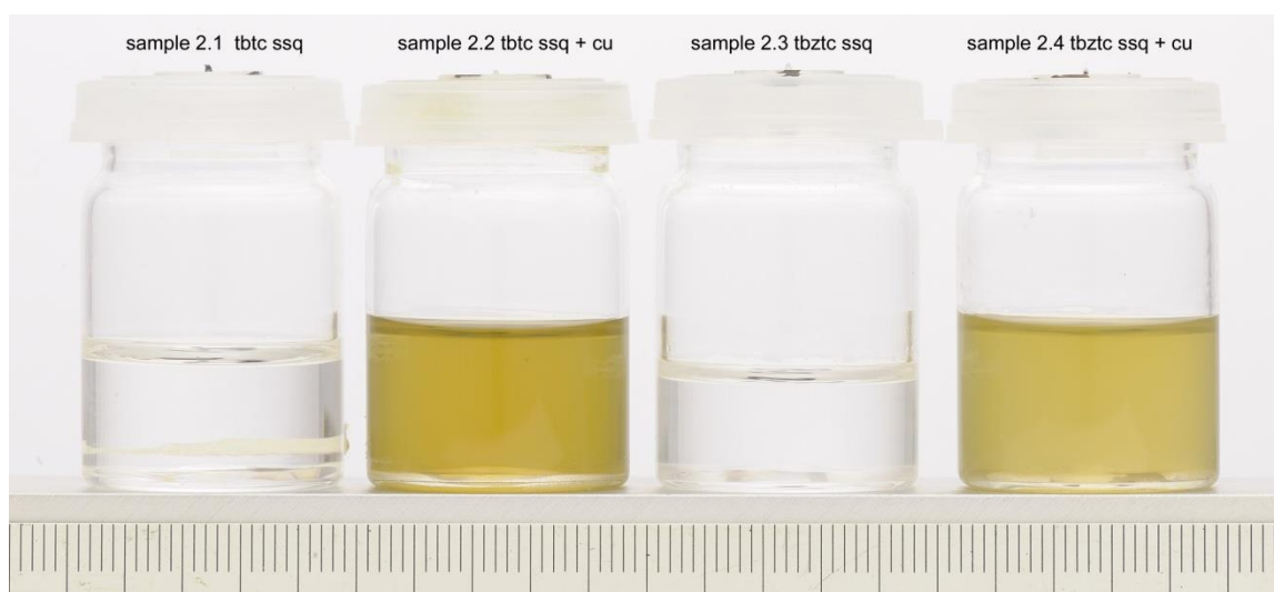
Figure 7 Photograph of dual and triple function silsesquioxane without and with exposure to copper nanoparticles. The coloured liquids have both been exposed to copper. The two dual functional silsesquioxane samples are on the left of the image, the two triple functional silsesquioxane samples are on the right of the image.
