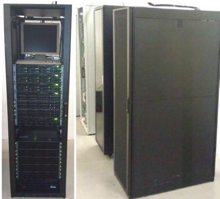
Figure 4: High performance cluster installed in Faculty of Mechanical Engineering (shared room for institutes IT equipment) cluster room, procured cluster consists of 32 computational nodes with 382 cores and more than 1800 GB RAM and headnode with distributed storage of 16 TB.
