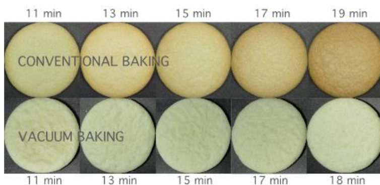
Figure 17. Biscuits baked at 180°C in conventional and vacuum oven
