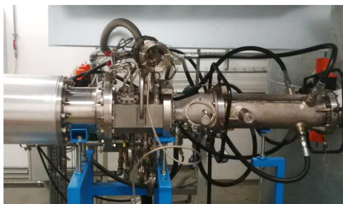
Figure 18: GE AVIO sector rig installed in the UNIFI facility
