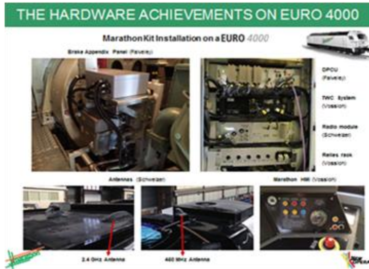
Figure 5 – Installation of MARATHON Kit on EURO 4000 Locomotive
