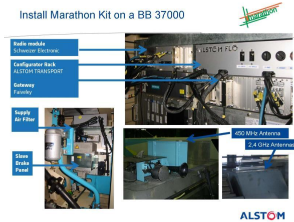
Figure 4 – Installation of MARATHON Kit on a BB 437000 Locomotive
