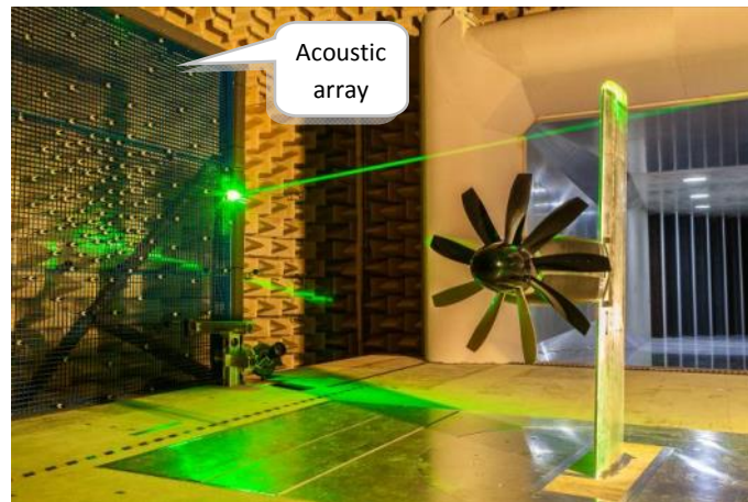
Figure 2 Picture of the wind tunnel model with laser light volume and acoustic array in the background, the return mirror is mounted on the array.
