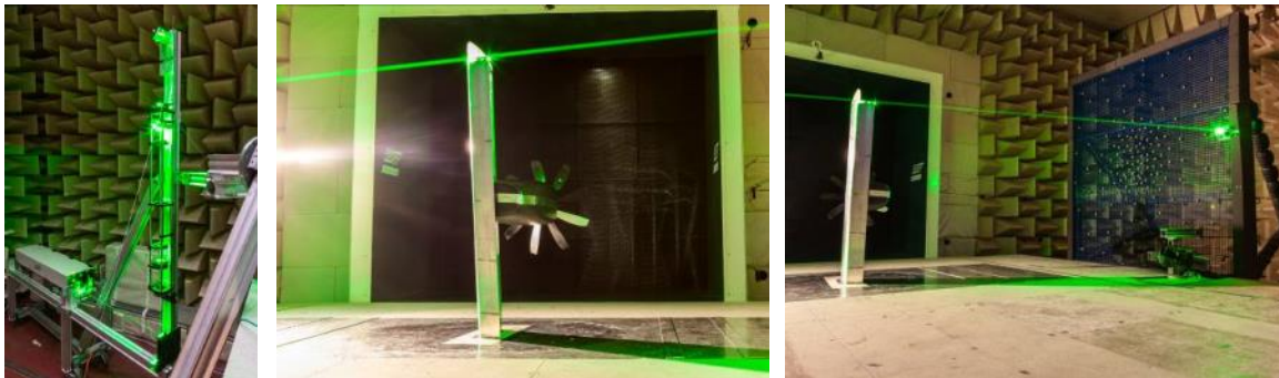
Figure 5 Laser light path from laser (left picture) along the flap (middle picture) towards the return mirror (right picture).
