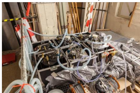
Figure 4 Multiple connected seeding generators and impactors supplying the seeding rake with particles.
