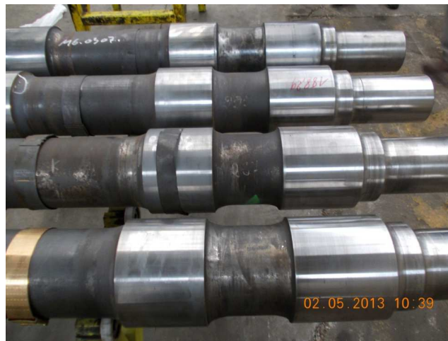
Figure 10 - A1N unpainted corroded axles from service.
