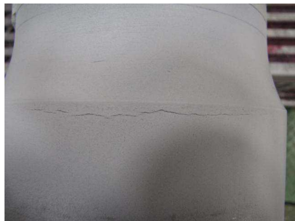
Figure 12 - Stair case fatigue test results of F4 A4T axles with a diameter ratio of 1,12. On the right side an example of surface crack found at the end of the test with MT inspection.
