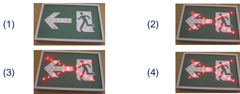
Figure 3: Negated signage design in operation depicting a single operation cycle.
