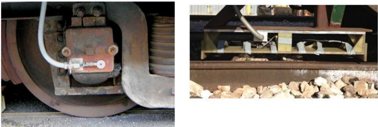
Figure 6 Accelerometer mounted on the wheel bearing (left picture) for short range rail measurement and Eddy Current sensor + accelerometer (right picture) for long range contour inspection
