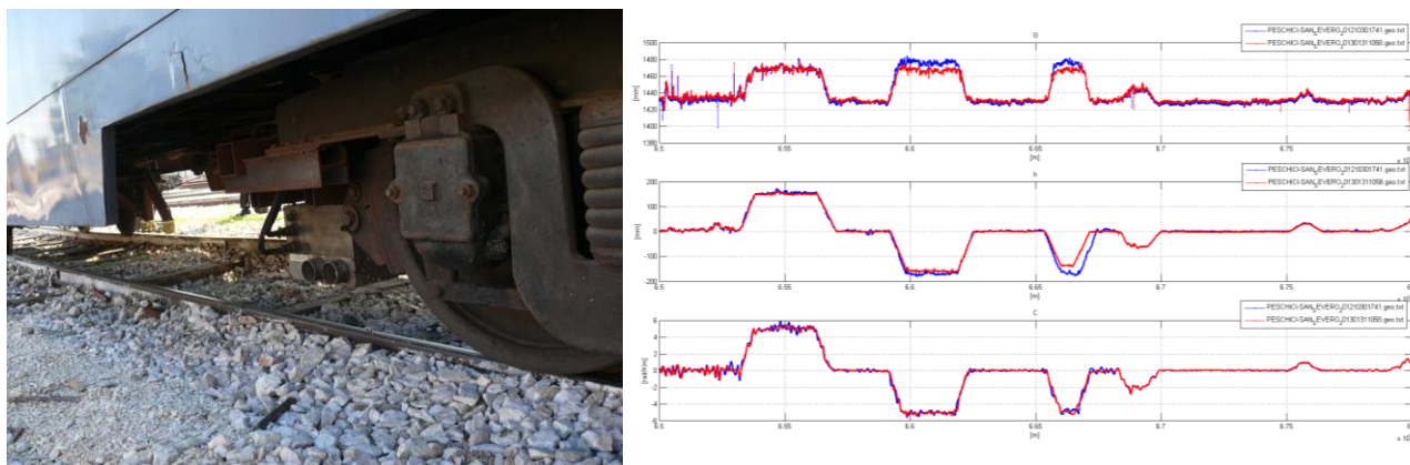
Figure 19 On left side, laser profiler and inertial pack mounted in the coach (Ferrovie del Gargano, Italy). On right side, output of the GUI software. Gauge, cant and curvature in section between KP 65.5 to 66.8. It shows evident track refurbishments.
