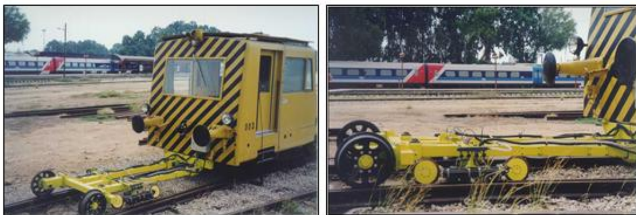
Figure 20 Slow speed rail inspector for in-service detection and evaluation of flaws.
