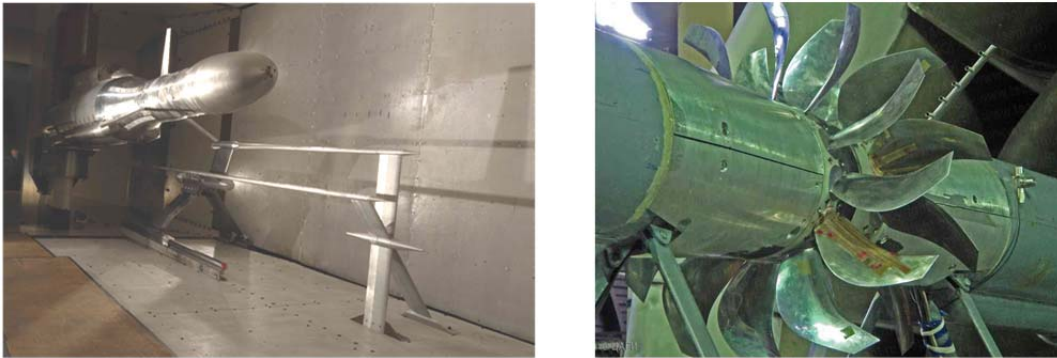
Figure 9: DREAM CROR designs in ARA (left) and TsAGI (right) wind tunnels
