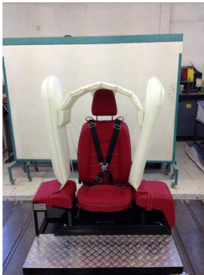
Fig. 23: Driver seat including four points belts and airbags (front view). A second C-shape configuration for the lateral airbags has also been studied and patented to contribute to protect the rear passengers (BIT17333 TO2014A000258).
