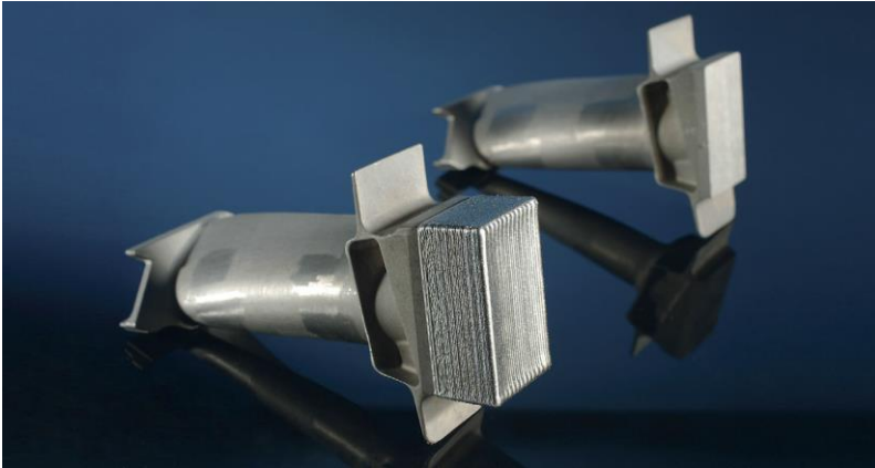
Figure 13: Extension of Blade Root out of LEK94 with Inconel 718
