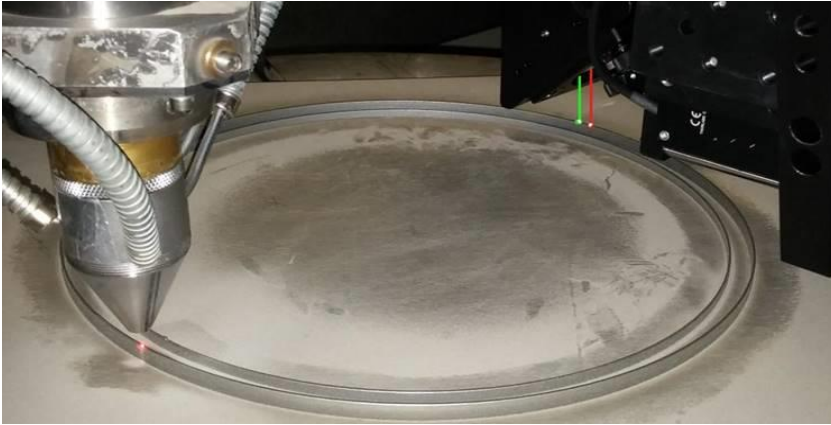
Figure 17: Relative positions of the LMD nozzle and LUT aperture on a circular wall deposit.
