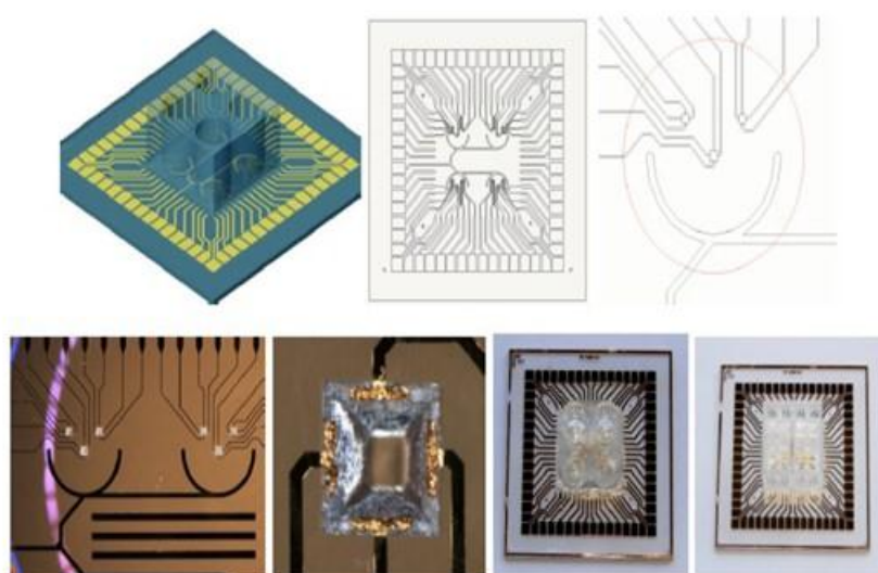
Figure Design and production of a 2x2 multiwell MCA for bioelectronic monitoring of hCMC.
