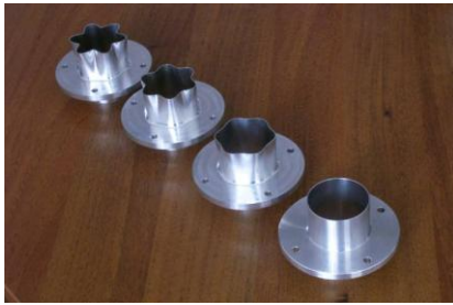
Figure 13 - Photographs of the corrugated nozzles and the circular nozzle with the equivalent area of the output cross section.
