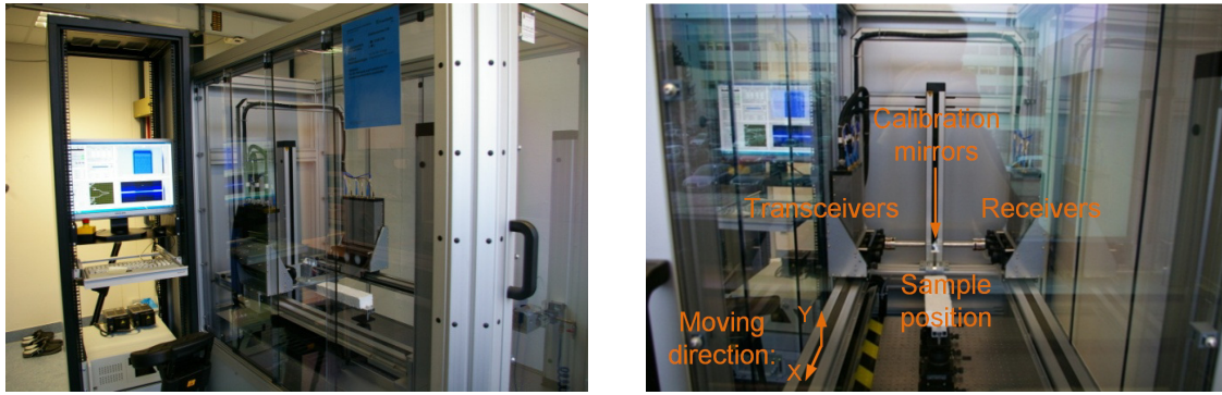
Figure 1- Photographs of the FMCW system. Left: side view with housing and control unit. Right: view from the front side showing the three transceivers and three receivers in transmission assembly. The z-direction between the transceivers and receivers is fixed
