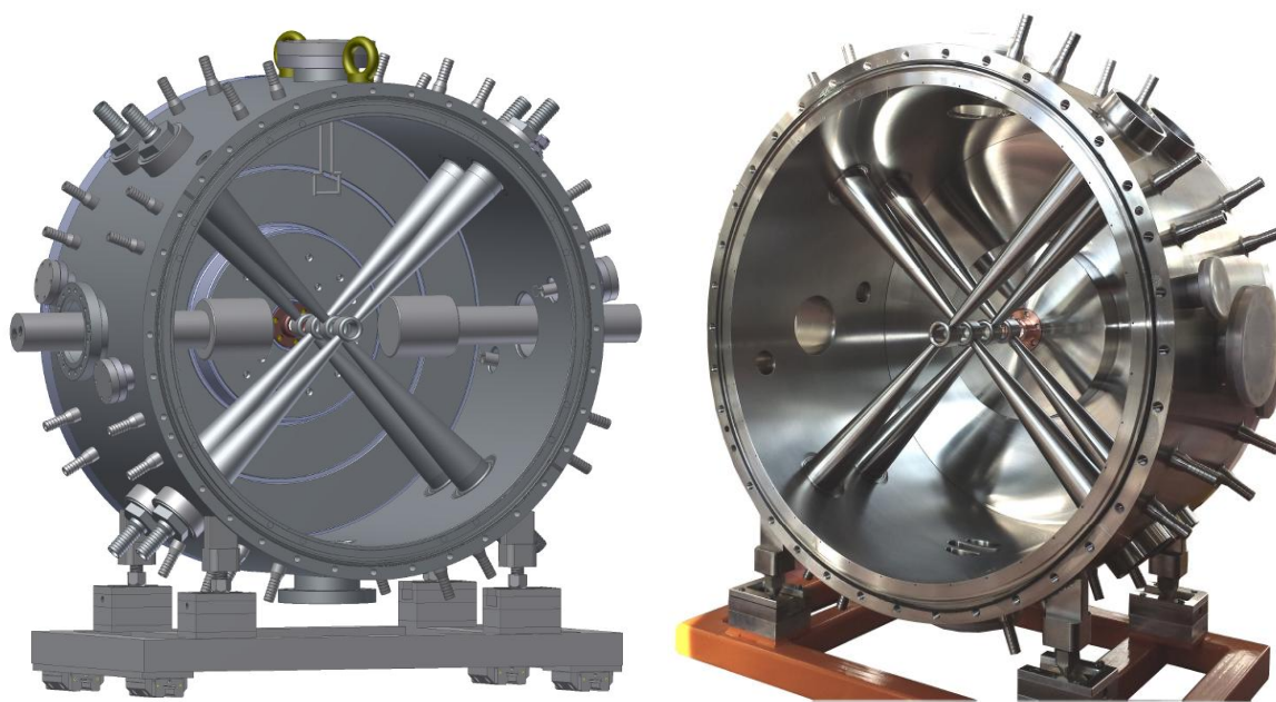
Figure 8: (Left) 3D plot of the complete CH-prototype cavity. (Right) Photograph of the manufactured CH-cavity before copper plating.
