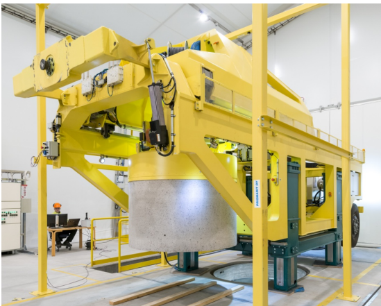
Figure 20. Bentonite installation machine at surface level test facility.
