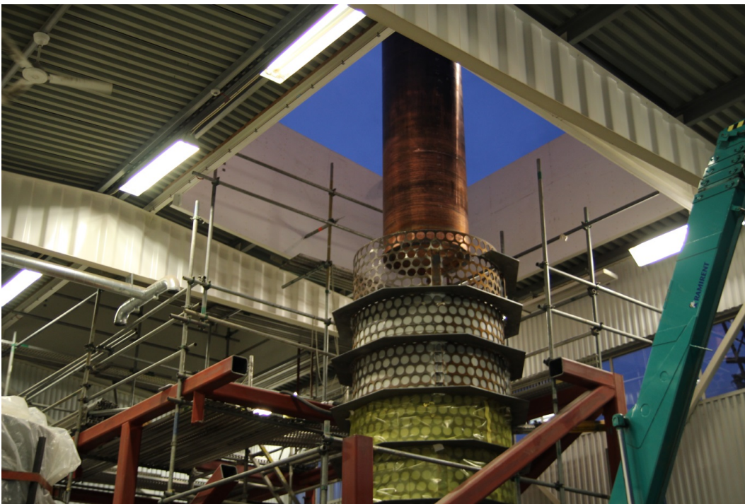
Figure 13. Canister being lowered into the Supercontainer during assembly. Stiffening plates for straightening the shell can be seen on its outer periphery.
