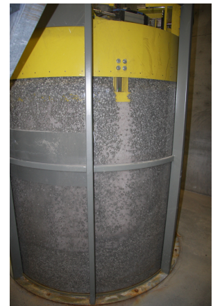
Figure: 20. Releasing of pellet into the gap between buffer and test hole wall
